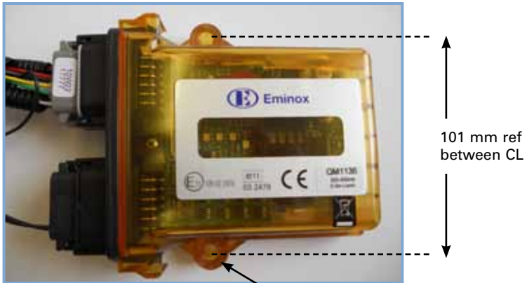
Figure 8 CPU Mounting Points
