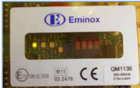
Figure 4 Max Pressure Display
