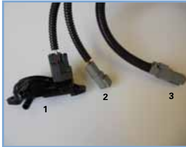
Figure 2 Detail of Sensor and Connectors
