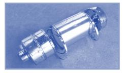
When the Filter Module is to be removed for servicing or exchange it may be possible to release it as a single unit by disconnecting its V-Clamps and easing away the adjacent Modules and pipe work.
