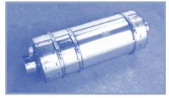
Your CRT<sup>®</sup> system may be removed as a complete unit by slackening Inlet Module and Outlet Module pipe retaining Band Clamps and dismantling the supporting brackets as necessary. Some installations like twin systems may require that one or more Modules be released first, in which case disconnect the V-Clamps and remove the CRT<sup>®</sup> system units individually.
