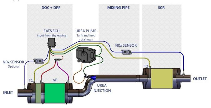
The EATS employ technologies such as a Diesel Oxidation Catalyst and Diesel Particulate Filter for PM regulation and a Selective Catalytic Reduction Catalyst for NOx control, as outlined below:
