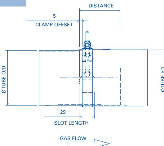
Figure 1: OD/ID Joint requirements
