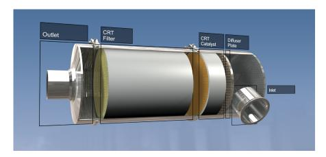
The wall-flow filter traps particulate matter, which is then oxidised by the  $\mathrm{NO}_2$  removing it from the filter. This chemical reaction takes place at normal exhaust temperatures, so the filter is cleaned by continuous regeneration during normal operation, without the need for any additives. Locating the catalyst before the filter leads to more effective filter regeneration.
