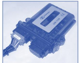
**ESI Warning System.** The ESI warning system consists of 3 coloured lights. Limits are set within the micro-processor by Eminox Ltd for a particular engine configuration and duty cycle. The ESI triggers the appropriate light illumination when a preset BP has been exceeded:
