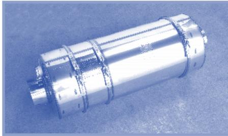
Your CRT® system may be removed as a complete unit by slackening Inlet Module and Outlet Module pipe retaining Band Clamps and dismantling the supporting brackets as necessary. Some installations like twin systems may require that one or more Modules be released first, in which case disconnect the V-Clamps and remove the CRT® system units individually.
